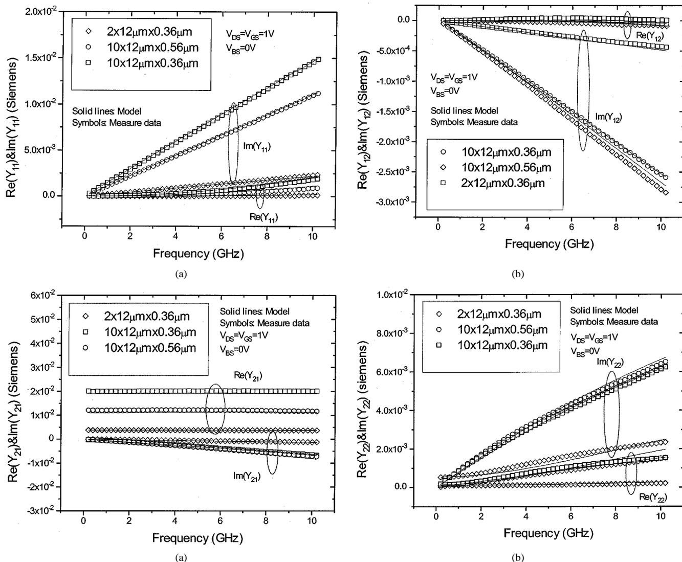
Fig. 2. Comparison of simulated and measured  $y$ -parameters (a)  $y_{11}$ ; (b)  $y_{12}$ ; (c)  $y_{21}$ ; and (d)  $y_{22}$  (both real part and imaginary part) versus frequency at  $V_{GS} = V_{DS} = 1V$  for several devices.
