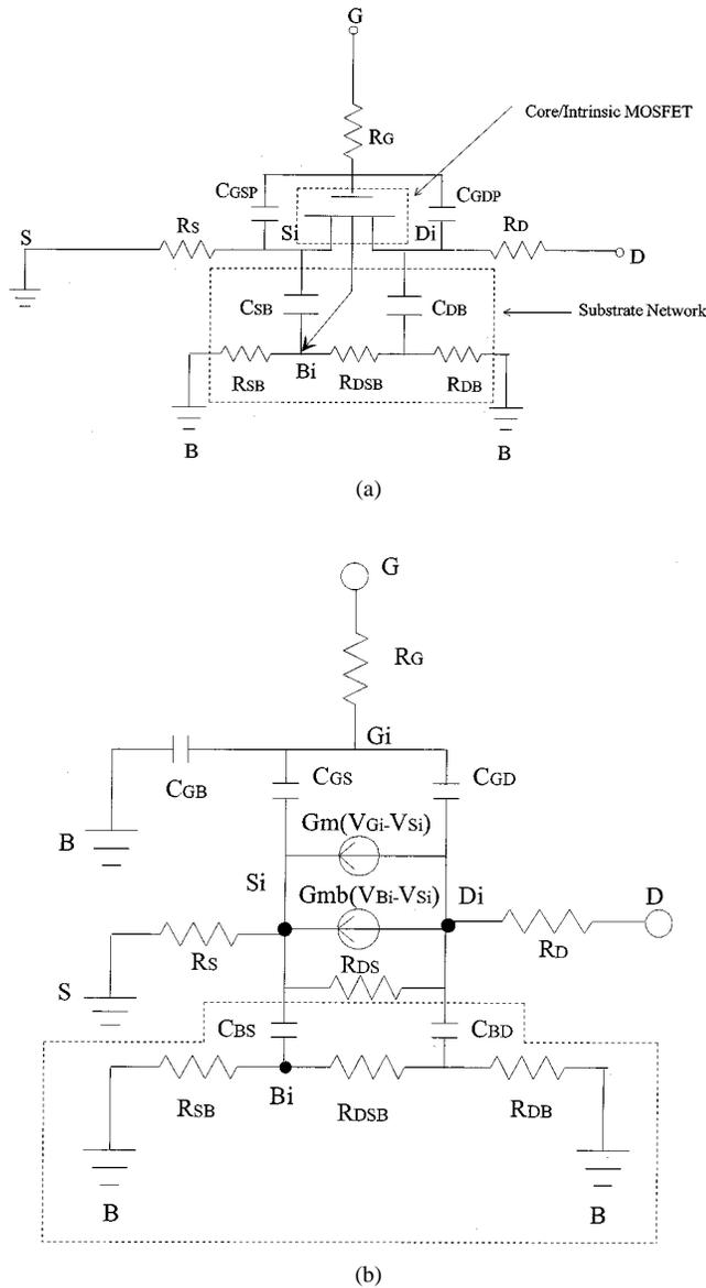
Fig. 1. (a) Schematic of the subcircuit model for a RF MOSFET and (b) an equivalent circuit of the subcircuit RF model in saturation regime.  $C_{GD} = C_{GDP} + C_{GDi}$  and  $C_{GS} = C_{GSP} + C_{GSi}$ , where  $C_{GDP} = C_{GD\text{total,extracted}} - C_{GD\text{intrinsic,simulated}}$  and  $C_{GSP} = C_{GS\text{total,extracted}} - C_{GS\text{intrinsic,simulated}}$ .
