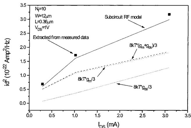
Fig. 9. Power spectral densities of channel thermal noise versus bias current of a  $0.36 \mu\text{m}$  n-channel MOSFET. They are extracted from the measured data and calculated from different channel thermal noise models.
