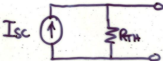
Circuit B cannot tell the difference between Circuit A, the Thevenin equiv and the Norton equiv.
