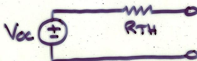
Circuit B cannot tell the difference between Circuit A and its Thevenin equivalent
