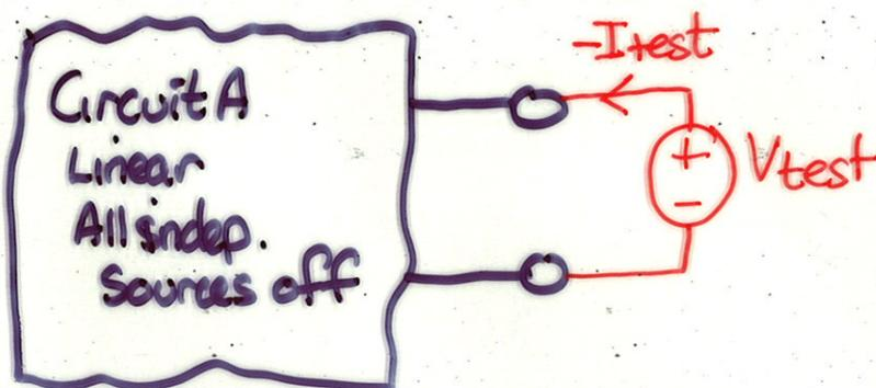
This is the equivalent resistance of the circuit
