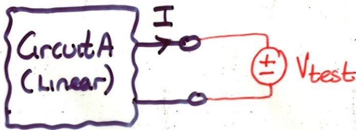
By superposition:  $I = I_{\text{test}} + I_{\text{sc}}$
