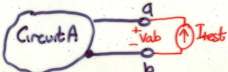
$$R_{Th} = \frac{V_{ab}}{I_{test}}$$
