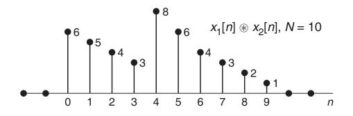
We note that in this case N > L + P - 1 (= 10), so the circular convolution does not exhibits time-aliasing, i.e., it is identical to the linear convolution of these sequences.
