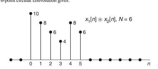
If *L* and *P* are the lengths of  $x_1[n]$  and  $x_2[n]$ , respectively, we note that N < L + P - 1 (= 10), so the circular convolution exhibits time-aliasing, i.e., it is not identical to the linear convolution of these sequences, shown below.
