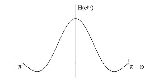
This system must have a zero on the unit circle of the z-plane, because its frequency response has a value of zero at  $\sim \pm \pi/2$ . Thus, the inverse of this system would have a pole on the unit circle, and consequently the inverse system *could not be stable*.
