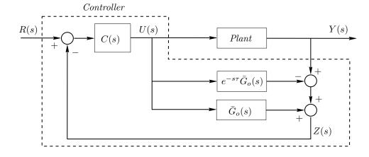
We can then design the controller using a a pseudo complementary sensitivity function,  $T_{zr}(s)$ , between *r* and *z* which has no delay in the loop. This would be achieved, for example, via a standard PID block, leading to:
