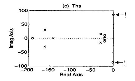
The corresponding frequency response shows a dip at the frequency of the imaginary axis zeros (*see next slide*).
