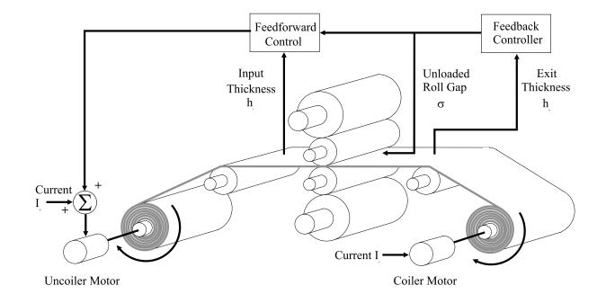
The above explanation suggests that a remedy might be to send a pulse of current to the uncoiler motor as soon as we adjust the roll gap, i.e. to use **FEEDFORWARD**. Indeed, one can show using the physics of the problem that tension fluctuations would be avoided by choosing the uncoiler current as
