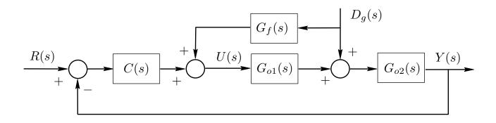
Figure 10.2: Disturbance feedforward scheme.
