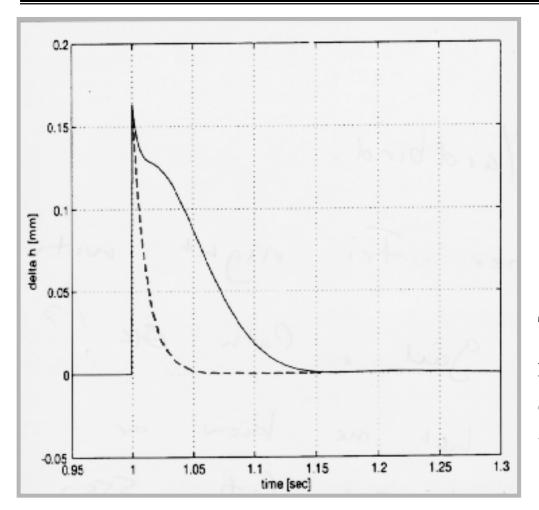
The dotted line represents the expected disturbance response whereas what is actually achieved is the solid line. Consider the schematic diagram shown on the next slide. We recall that the physical explanation for the hold-up effect is as follows:
