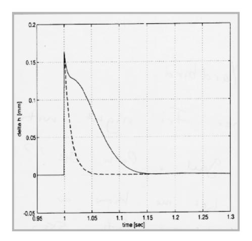
Recall that the solid line was the best that could be achieved with a single degree of freedom control whereas using feedforward we can achieve the dotted line. The above example delivers an important message in solving tough control problems. Specifically, one should look out for architectural changes which may dramatically change a difficult (*or maybe impossible*) problem into an easy one.
