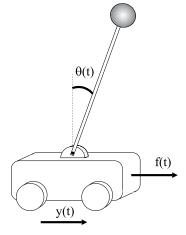
Figure 3.5: Inverted pendulum
