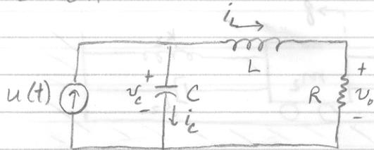
The state of the system can be described by a set of state variables  $(x_1, x_2) = (v_c(t), i_L(t))$
