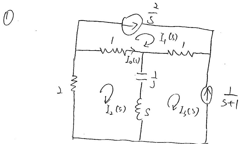
$$\textcircled{1} \text{ Loop equations: } (2 + 1 + \frac{1}{s} + s) I_2(s) = I_1(s) + (\frac{1}{s} + s) I_3(s)$$
