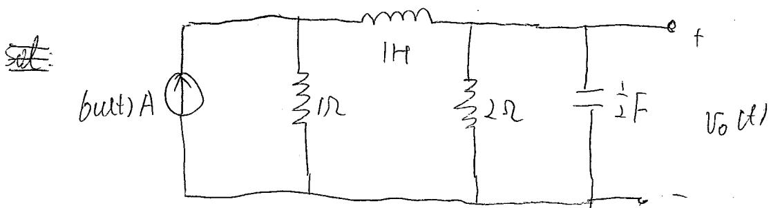
sol: For  $t > 0$ , the input is DC, all voltages and currents will become DC as well, so.  $V_c \rightarrow 0$  and  $i_L \rightarrow 0$  as  $t \rightarrow \infty$ .
