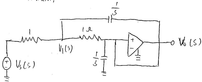
$$1) \frac{V_s(s) - V_1(s)}{1} = \frac{V_1(s) - V_o(s)}{\frac{1}{s}} + \frac{V_1(s)}{1 + \frac{1}{s}}$$
