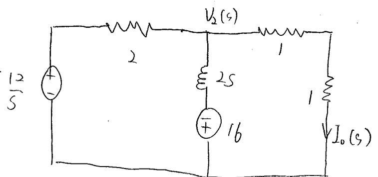
$$1) \text{ KCL at } V_2: \quad \frac{\frac{12}{s} - V_2(s)}{2} = I_o(s) + \frac{V_2(s) + 16}{2s}$$
