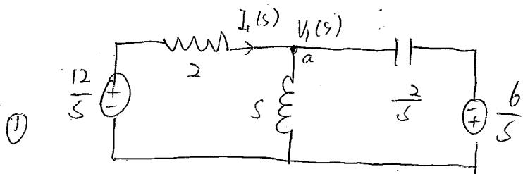
$$\textcircled{2} \text{ KCL at } a: \frac{\frac{12}{s} - V_1(s)}{\frac{1}{s}} = \frac{V_1(s)}{s} + \frac{V_1(s) + \frac{6}{s}}{\frac{2}{s}}$$
