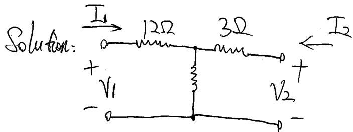
$$Y_{11} = I_1 / V_1 \Big|_{V_2=0} = \frac{1}{12 + (6//3)} = \frac{1}{14} S.$$
