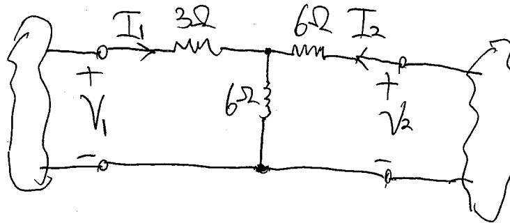
$$\text{Solution: } \Upsilon_{11} = \frac{I_1}{V_1} \Big|_{V_2=0} = \frac{1}{3 + (6//6)} = \frac{1}{6} \text{ S.}$$
