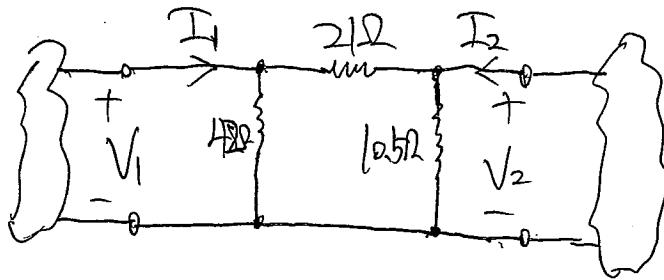
$$\text{So } Z_{11} = \frac{V_1}{I_1} \Big|_{I_2=0} = 4\Omega \parallel (2 + 1.5) = 1.8\Omega$$
