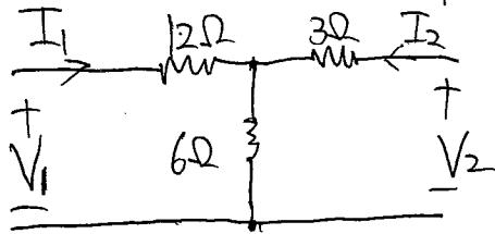
$$\text{Solution: } A = \frac{V_1}{V_2} \Big|_{I_2=0} \Rightarrow V_2 = \frac{6}{18} V_1 \Rightarrow A = 3$$
