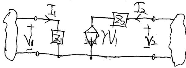
$$\text{Solution: } A = \frac{V_1}{V_2} \Big|_{I_2=0} \Rightarrow V_2 = -rV_1 \Rightarrow A = -\frac{1}{r}$$
