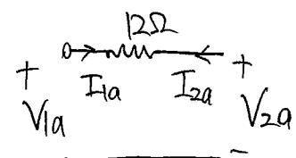
$$A_a = \frac{V_1}{V_2} \Big|_{I_2=0} = 1$$
