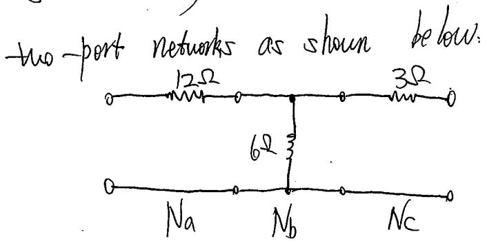
Solution: Network consists of 3 two-ports.
