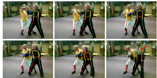
Fig. 8. Failure cases are pointed by red arrows. The pose of elbow and head are unable to be detected because of occlusion and image blurry.
