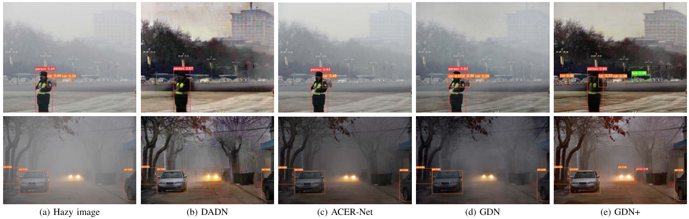
Fig. 11. Task-Driven Evaluation. YOLOv3 is leveraged to detect objects on real-world hazy images and the dehazing results from different methods.
