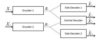
Fig. 1. Block diagram of robust distributed source coding.
