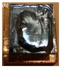
Fig. 5. Fracture images of Si/glass bonded using (a) the RIE plasma activated anodic bonding and (b) the hybrid plasma bonding at 200 °C.
