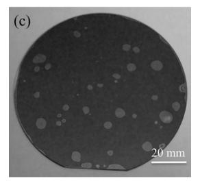
**Fig. 2.** Optical images of Si/glass wafers anodically bonded at temperature of (a) 100, (b) 150 and (c) 200 °C. Anodic bonding voltage of 1 kV was applied for 10 min.
