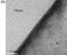
Fig. 6. HRTEM images with (a) low and (b) high magnifications. A  $\sim$ 353 nm thick bright depletion layer in the glass and an indistinct dark edge of Si near the interface are observed.
