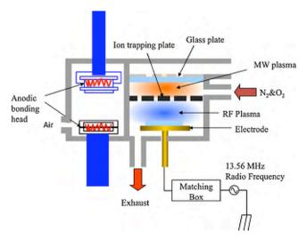
Fig. 1. Hybrid plasma bonding system.
