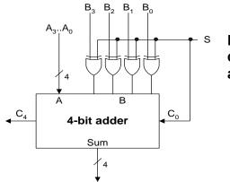
Figure 3 – Circuit for questions 7 to 11. Note,  $c_0$  is carry in and  $c_4$  is carry out for the 4-bit adder.
