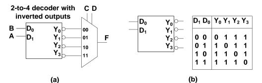
Figure 2 – (a) Circuit for question 5. (b) Truth table of the decoder with inverted outputs
