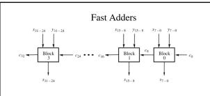
Figure 5.17. A hierarchical carry-lookahead adder with ripple-carry between blocks.
