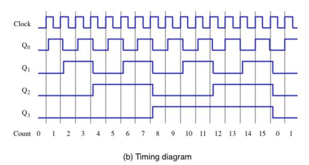
Figure 7.22. A four-bit synchronous up-counter.
