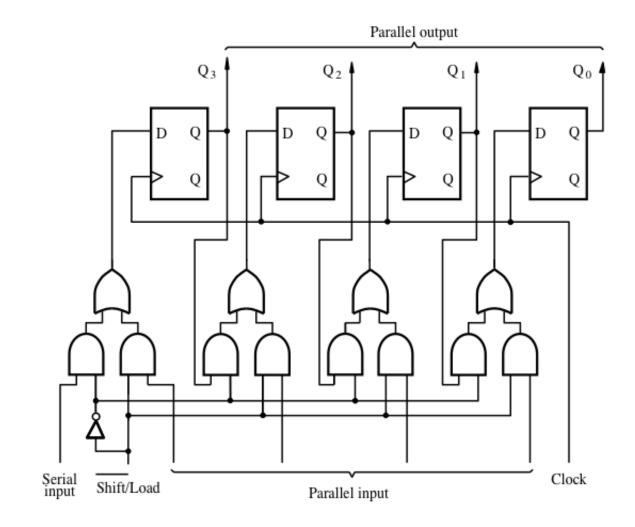
Figure 7.19. Parallel-access shift register.
