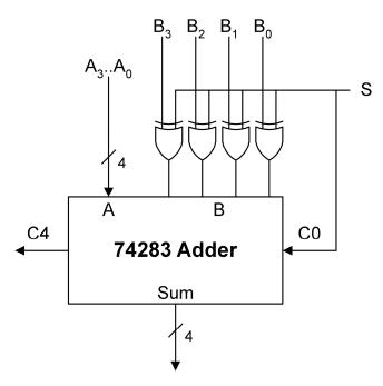
The adder/subtractor may be used to take the 2's complement of an input number B by setting A=0000 and S=1. Try this for several values. In the last circuit, we use this feature to take the 2's complement of a number if it is negative in order to provide input to a display.
