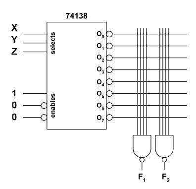
Draw the truth table for a full adder, and "program" this circuit such that the output  $F_1$  represents the sum S and output  $F_2$  represents the carry C. Mark every intersection where there is a connection with an "X". Build the circuit and verify its operation.
