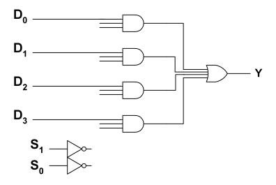
2. The n-bit binary decoder generates an output corresponding to each of the  $2^n$  minterms of the input. Complete the drawing of the circuit shown below to implement a 2-to-4 line decoder with inputs  $S_0$ ,  $S_1$ , LO-true outputs  $D_0$ ... $D_3$  and a single LO-true enable. Build the circuit and verify its function table.
