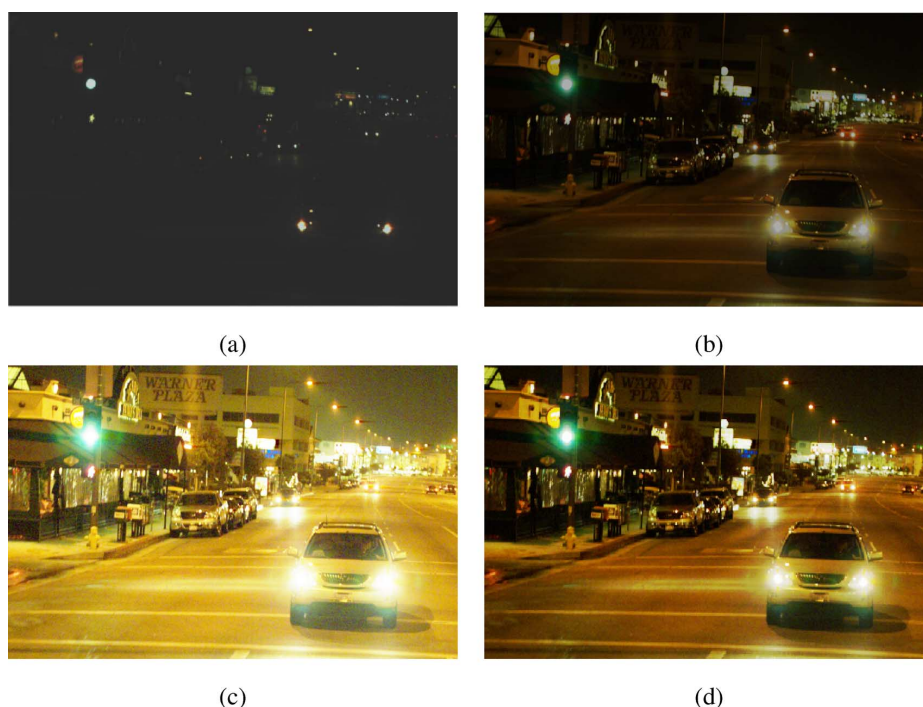
Fig. 4. (a) Original image before Gamma correction. (b) After Gamma correction. (c) Gamma correction followed by histogram equalization. (d) Joint Gamma correction and contrast-tone optimization by the proposed OCTM method.
