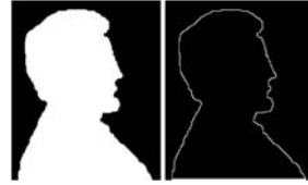
FIGURE 9.14 (a) A simple binary image, with 1's represented as white. (b) Result of using Fig. 9.13(b) with the structuring element on Fig. 9.13(a).
