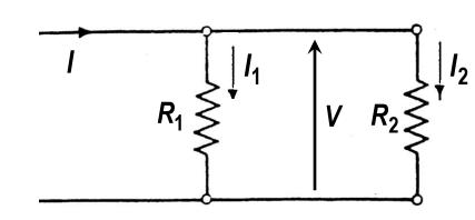
$$\begin{split} V &= I \frac{R_1 \ R_2}{R_1 + R_2} \\ I_1 &= \frac{V}{R_1} = \frac{I \ R_2}{R_1 + R_2} \,, \quad I_2 = \frac{V}{R_2} = \frac{I \ R_1}{R_1 + R_2} \,, \quad \frac{I_1}{I_2} = \frac{R_2}{R_1} \end{split}$$
