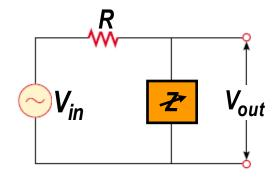
$$A_{v} \equiv \text{voltage gain} \equiv \frac{V_{out}}{V_{in}} = \frac{Z}{Z+R}$$
