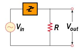
$$A_{\nu} \equiv \text{voltage gain} \equiv \frac{V_{out}}{V_{in}} = \frac{R}{R+Z}$$
