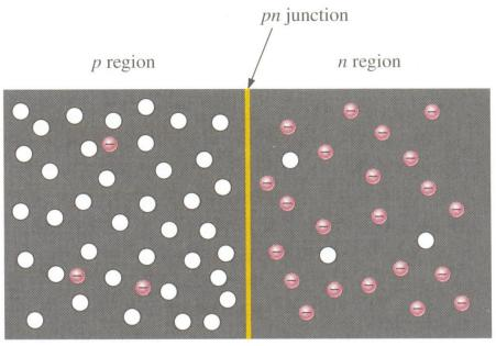
The <u>diode (pn junction)</u> is formed by dopping a piece of intrinsic silicon, such that a p-type region is adjacent to a n-type region.
