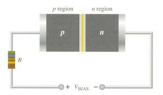
The +ve side of  $V_{\text{BIAS}}$  is connected to the *p*-type.
