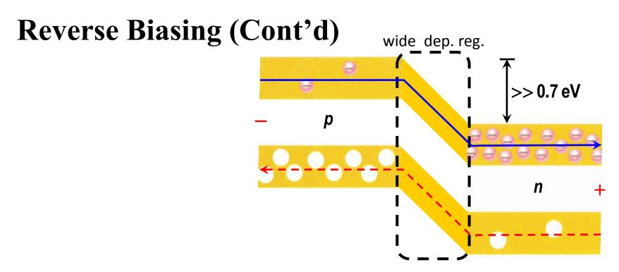
The energy band shifts up in the region connected to the -ve side of the battery and shifts down in the other region connected to the +ve side, which deepen the energy hills.
