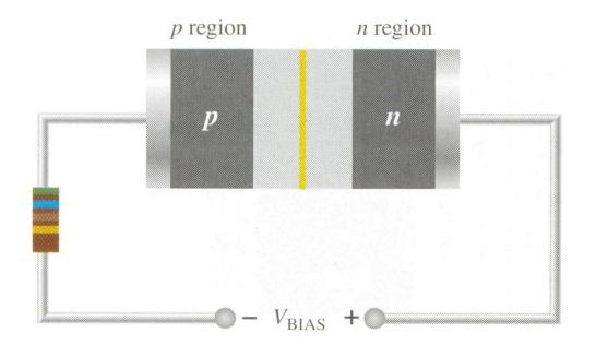
The +ve side of  $V_{\text{BIAS}}$  is connected to the *n*-type.
