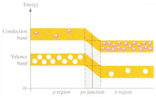
Due to this process of energy transfer, the energy bands of the n-type are shifted down, and those of the p-type are shifted up. This difference in energy bands, which is proportional to the *barrier potential (0.7V)*, prevents further diffusion of electrons.
