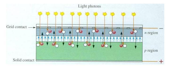
Incident solar energy is composed of *photons* (energy packets) whose wavelengths fall within *visible light* range (350 nm till 750 nm)
