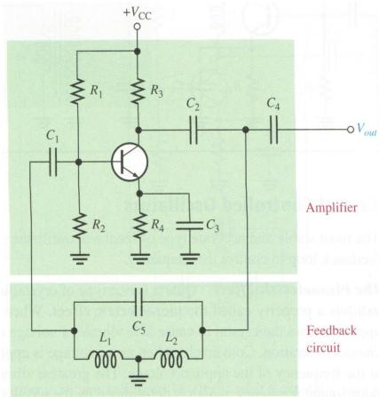
$$B = \frac{V_f}{V_{out}} \cong \frac{-I X_{L1}}{I X_{L2}} = -\frac{X_{L1}}{X_{L2}} = -\frac{2\pi f_r L_1}{2\pi f_r L_2} = -\frac{L_1}{L_2}, \quad A_v = \frac{1}{B} = -\frac{L_2}{L_1}$$
