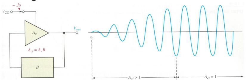
the power supply turn-on transients generate all frequency components in the oscillator loop
