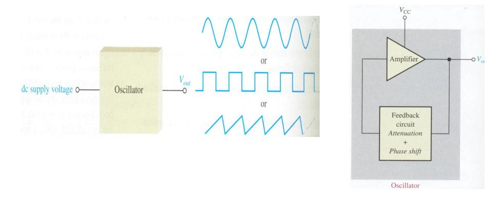
A feedback oscillator is created by forming a closed loop consisting of an amplifier with voltage gain  $(A_v)$  and a feedback circuit with attenuation (B).
