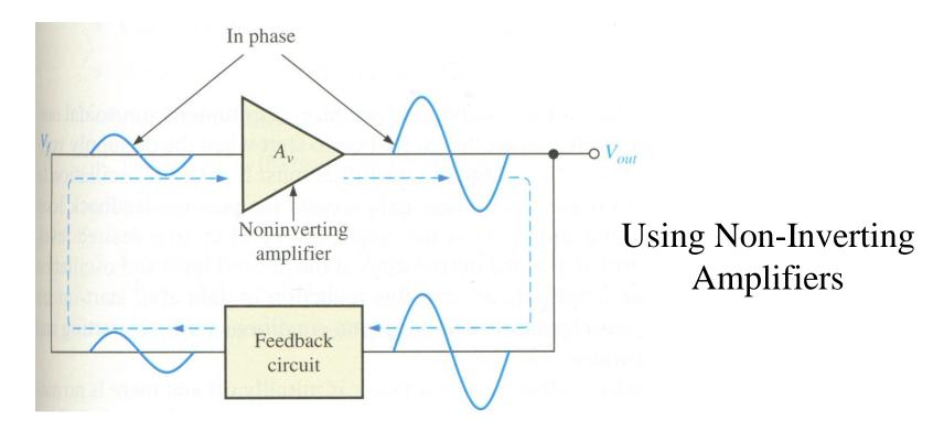
$A_{cl} \equiv$  voltage gain around the closed loop =  $A_{v} B = 1$
