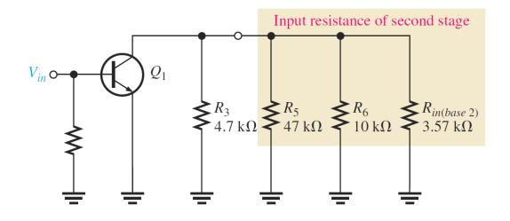
$$Rc_1 = 4.7 \text{ K}\Omega//47 \text{ K}\Omega//10 \text{ K}\Omega//3.57 \text{ K}\Omega = 1.63 \text{ K}\Omega$$
