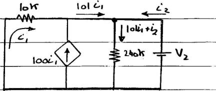
$$\text{We have } V_2 = 240k (10i_1 + i_2)$$
