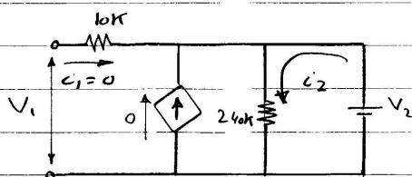
$$\therefore h_{12} = V_1 / V_2 \quad , \quad h_{22} = i_2 / V_2$$
