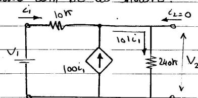
$$V_2 = 240k \cdot 10i_1 \Rightarrow g_{21} = \frac{24.24 \times 10^6 i_1}{24.25 \times 10^6 i_1}$$
