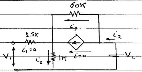
$$\Rightarrow Z_{22} = V_2 / i_2 = 61 k \Omega$$
