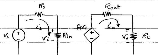
$$\text{a. } A_V = \frac{V_o}{V_s} \quad \text{but } V_o = R_L i_o = \frac{A V_i}{R_L + R_{out}} \cdot R_L$$
