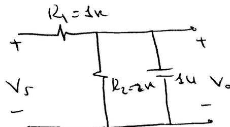
$$V_o = \frac{Z_2}{Z_1 + Z_2} V_s = \frac{R_2 \times \frac{1}{sC}}{R_1 + \frac{R_2 + \frac{1}{sC}}{R_2 + \frac{1}{sC}}} V_s = \frac{R_2}{1 + sCR_2} V_s$$
