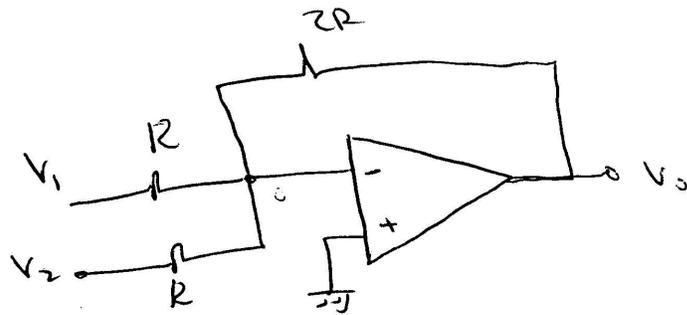
$$\begin{aligned} V_o &= -2(V_1 + V_2) \\ V_o &= A_{CM} \left( \frac{V_1 + V_2}{2} \right) + A_d (V_1 - V_2) \\ \therefore A_d &= 0 \\ A_{CM} &= -4 \end{aligned}$$
