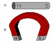
Two of the most familiar types of magnets are the bar magnet (A) and the horseshoe magnet (B). Their names reflect their physical shape.
