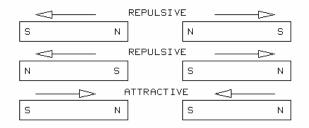
These arrows represent the direction of the attractive or repulsive magnetic forces. If a pole of one magnet is moved toward the similar pole of a second magnet (north to north or south to south), the magnets repel, or push away from, each other. If a pole of one magnet is moved toward the opposite pole of a second magnet (north to south), the magnets attract, or pull toward, each other. This relationship can be stated simply: opposite poles attract and like poles repel.
