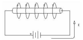
**Electromagnetism** is a form of magnetism created when current flows through a conductor. When current is present, it generates a magnetic field around the conductor similar to that of a permanent magnet. When current is removed, the magnetic field disappears.
