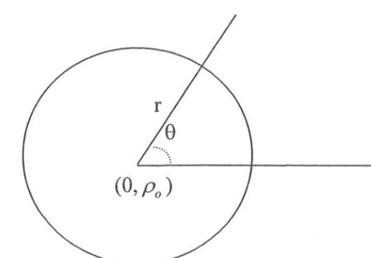
Flux per turn  $\Psi = \int_{r=0}^a \int_{\theta=0}^{2\pi} \frac{\mu NI}{2\pi\rho_o} \left(1 - \frac{r \sin \theta}{\rho_o}\right) r dr d\theta = \frac{\mu NI}{2\pi\rho_o} \frac{a^2}{2} (2\pi)$
