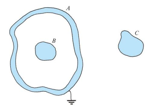
by surrounding a region by a grounded conductor, this region becomes electromagnetically isolated from any fields or charges outside the shield
