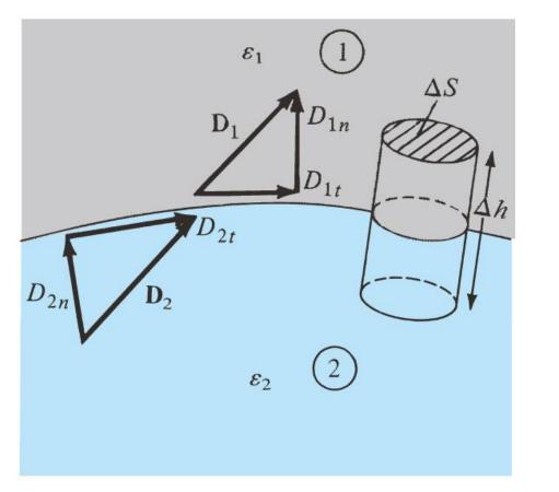
applying Gauss' law as  $\Delta h \rightarrow 0$  $D_{1n}\Delta s - D_{2n}\Delta s = \rho_s \Delta s$  $D_{1n} - D_{2n} = \rho_{s}$ if  $\rho_s = 0$  $\mathcal{E}_1 E_{1n} = \mathcal{E}_2 E_{2n}$  $E_{2n} \stackrel{\checkmark}{=} \frac{\mathcal{E}_1}{\mathcal{E}_2} E_{2n}$
