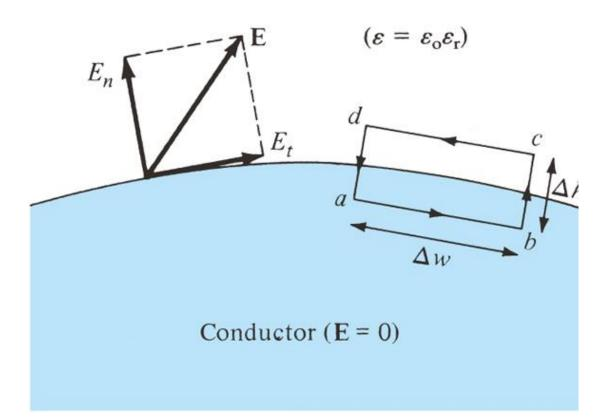
because there is no field inside the conductor,  $E_t=0$  at the dielectricconductor interface
