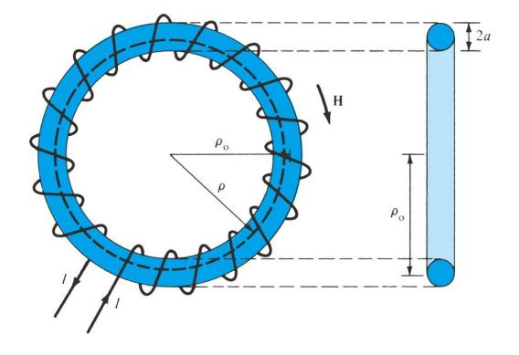
$$\Rightarrow H_{\phi} 2\pi\rho = N \cdot I \quad \Rightarrow H_{\phi} = \frac{N \cdot I}{2\pi\rho}, \ \rho_{1} \le \rho \le \rho_{2}$$
