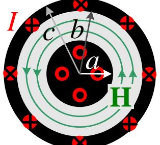
$$H_{\phi} = \frac{I\rho}{2\pi a^2}, \text{ A/m}$$
