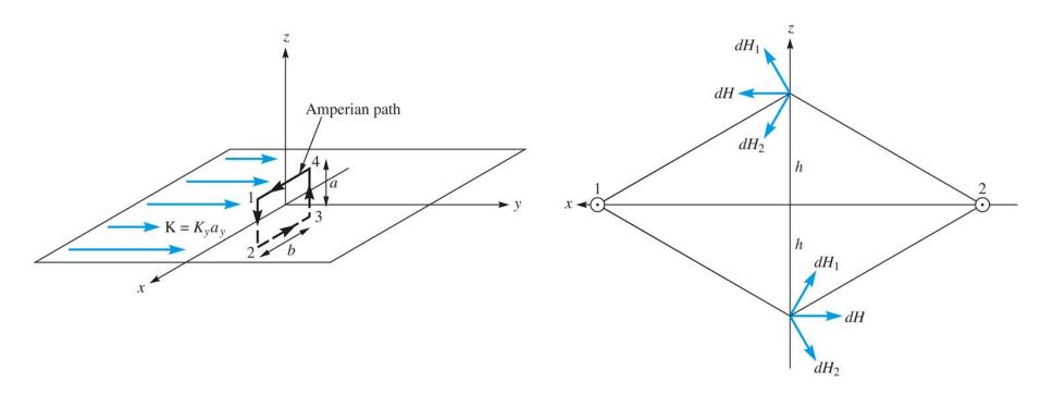
because of symmetry, magnetic field will be in the x direction and should depend only on z!
