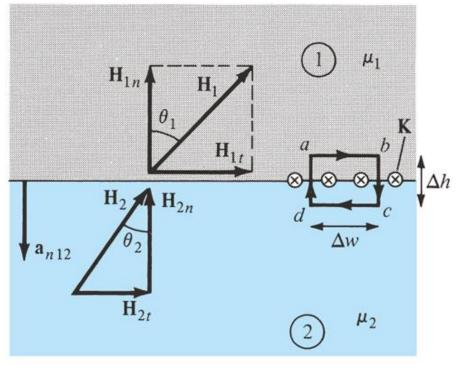
$\mathbf{H}.d\mathbf{l} = I$ as  $\Delta h \rightarrow 0$ , we have  $K\Delta w = H_{1t}\Delta w - H_{2t}\Delta w$  $H_{1t} - H_{2t} = K$ in general  $(\mathbf{H}_1 - \mathbf{H}_2) \times \mathbf{a}_{n12} = \mathbf{K}$
