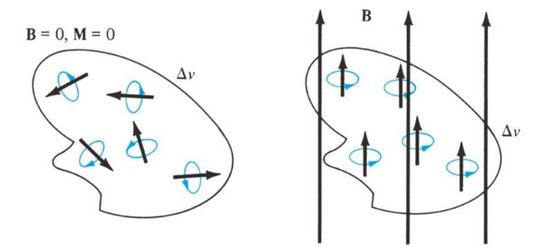
external magnetic field creates torque on all atomic magnetic dipoles and align them along its direction
