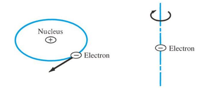
electron spinning around the nucleus is equivalent to a small current loop with a magnetic moment
