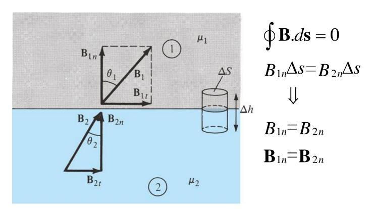
normal component of the magnetic flux density vector is continuous across any interface
