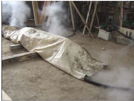
Fig. 6 Bending of wood plate
