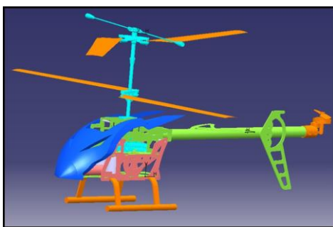
Fig. 5 - Example of CAD project modeling results: Remote controlled toy-helicopter (CATIA model)
