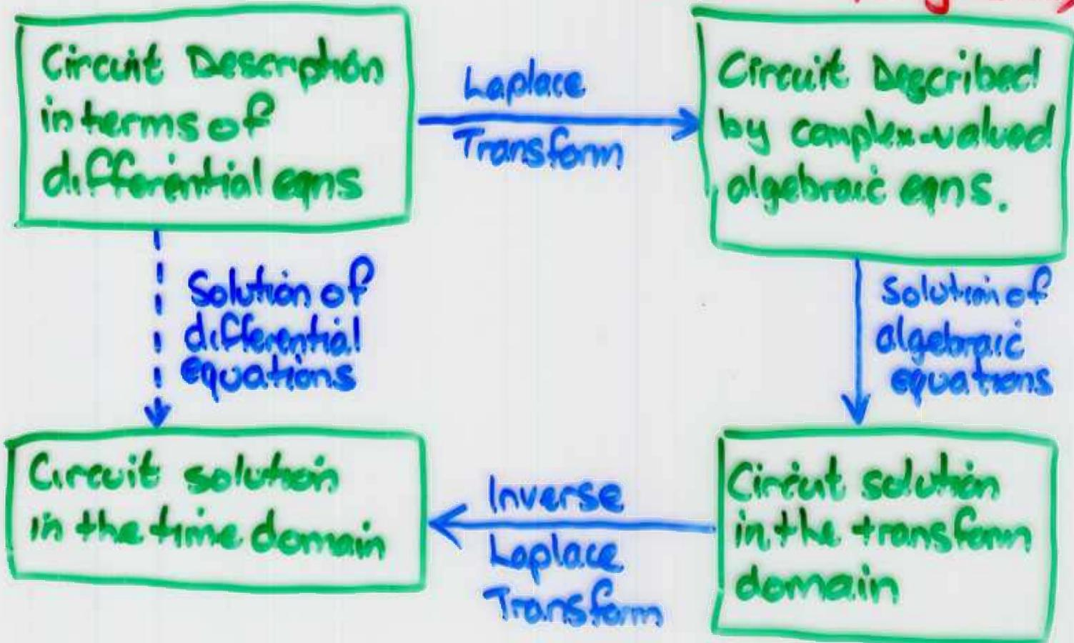
A similar diagram applies for steady-state analysis of circuits excited by sinusoidal signals. The "transform" in that case is the phasor.
