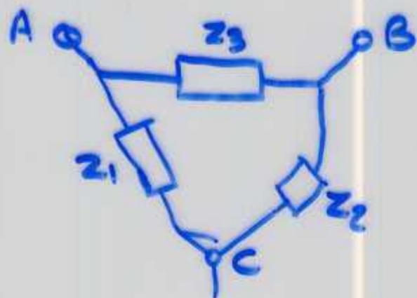
We can build a "Y-equivalent model" for this circuit, but first we analyze it in general.
