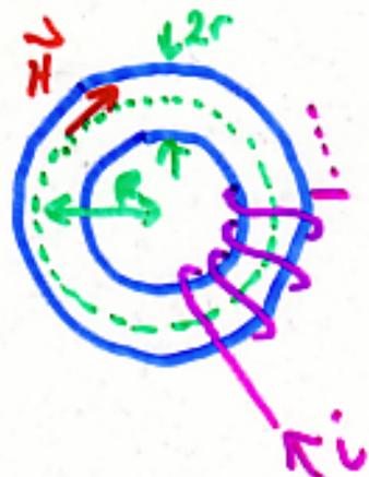
$N$  uniformly spaced turns on a bagel shaped core
