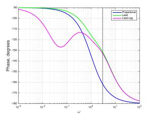
Observe additional phase from lead compensator and improved phase margin. By design, lead-lag does not reduce this much.
