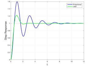
Note reduction in overshoot (larger damping ratio), and shorter settling time (wider closed-loop bandwidth)
