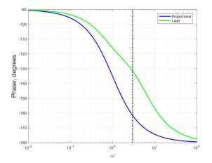
Observe additional phase from lead compensator and improved phase margin
