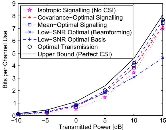
Fig. 3. Achievable rates versus transmitted signal power for different transmission schemes over a correlated channel model with Kronecker-structured covariance and nonzero mean.
