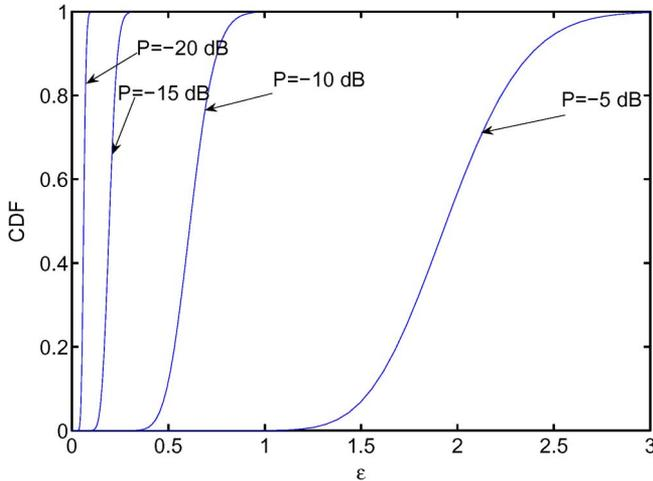
Fig. 2. CDF of  $P\lambda_{\max}(T)\lambda_{\max}(R)\lambda_{\max}(R^{-1}\check{H}\check{H}^\dagger)$  for different values of  $P$ .
