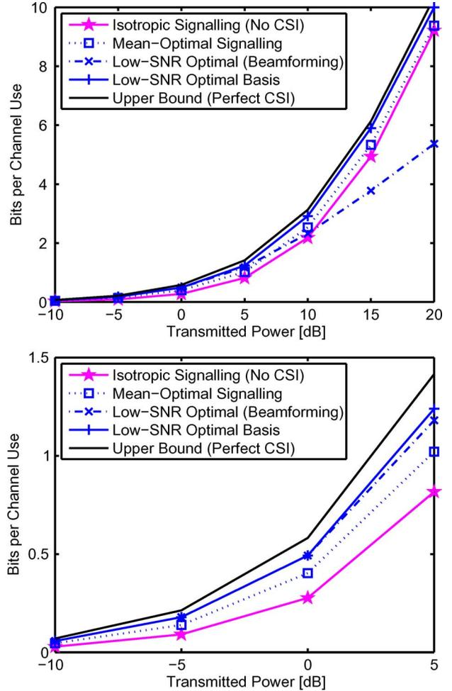
Fig. 1. Achievable rates versus transmitted signal power for different transmission schemes over an arbitrarily correlated channel model with nonzero mean. The signaling schemes are as follows: isotropic signaling (Strategy 1), mean-optimal signaling (Strategy 2), optimal signaling for low SNRs (beamforming, Strategy 3), and signaling along low-SNR optimal basis (Strategy 4). The lower figure provides the details of the low-SNR region of the upper figure.
