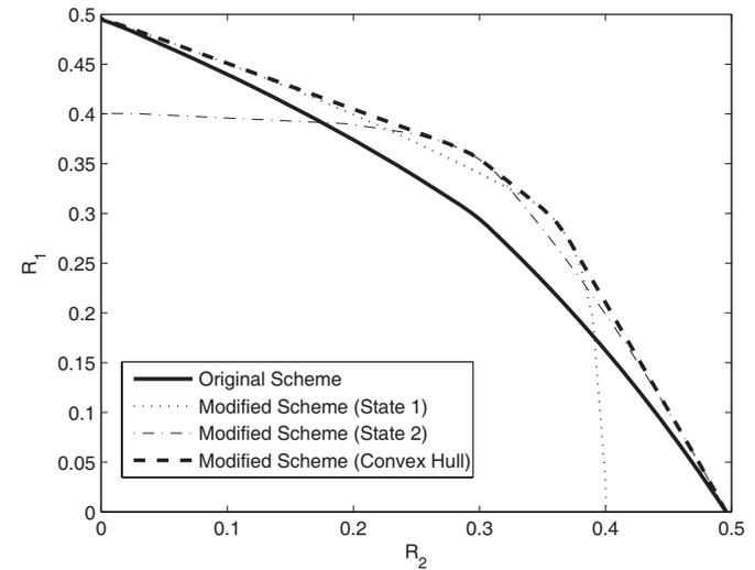
Fig. 8. Achievable rate region of the modified orthogonal AF scheme in the case of symmetric direct channels considered in Fig. 4.
