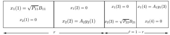
Fig. 2. A frame of the orthogonal half-duplex amplify-and-forward cooperation scheme under consideration.
