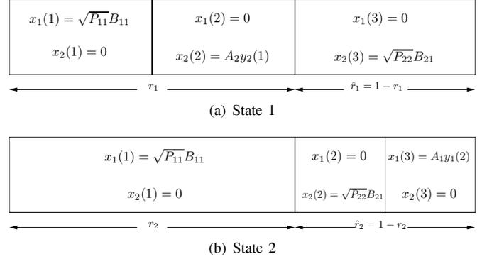
Fig. 3. One frame of each state of the proposed modified orthogonal amplify-and-forward cooperation scheme.
