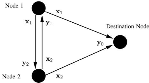
Fig. 1. Transmitted and received signals of the cooperative channel.
