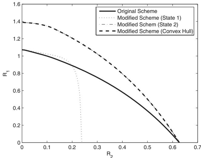
Fig. 9. Achievable rate region of the modified orthogonal AF scheme in the case of asymmetric direct channels considered in Fig. 6.
