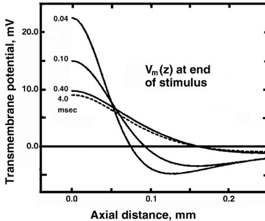
**Figure 7.9.** Spatial Distribution of Transmembrane Potential,  $v_m(z)$ , at the End of the Stimulus. Each curve is labeled with the duration of the stimulus. The source–fiber distance is 0.10 cm. In each case the stimulus magnitude is for a just subthreshold response. From Barr RC, Plonsey R. 1995. Threshold variability in fibers with field stimulation of excitable membranes. *IEEE Trans Biomed Eng* 42:1185–1191. Copyright ©1995 IEEE.
