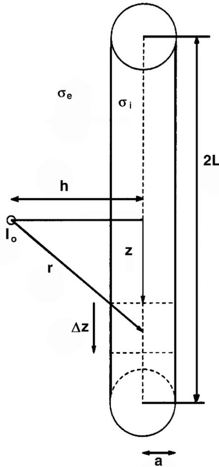
**Figure 7.5.** Geometry of Source and Fiber. A single current point source of magnitude  $I_0$  is placed at a distance  $h$  from a circular cylindrical fiber of length  $2L$ . The extracellular region is unbounded, uniform, and has a conductivity  $\sigma_e$ . The fiber radius is  $a$  and its intracellular conductivity is  $\sigma_i$ . The fiber's centerline lies along the coordinate  $z$  axis. The length is divided into elements  $\Delta z$  for numerical calculations.
