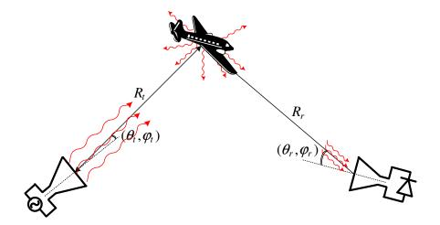
The target is represented by its RCS  $\sigma$ , which is used to calculate the captured power  $P_c = \sigma W_t$  (W), which, when scattered isotropically, gives the power density measured by the receiving antenna. The density of the scattered power at the Rx antenna is
