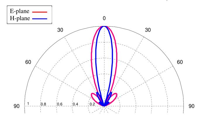
For electrically large apertures, the main beam is narrow and the  $(1-\sin^2\theta\cos^2\varphi)^{1/2}$  in (17.51) is roughly equal to 1 for all observation angles within the main beam. That is why, in the theory of large apertures and arrays, it is assumed that the amplitude pattern is simply
