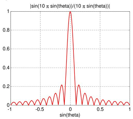
Notice that the side-lobe level in both patterns is the same although the size of the aperture is different in the x and y directions ( $L_x = 20\lambda$ ,  $L_y = 10\lambda$ ). This is due to the first minor maximum of the function  $|\sin u/u| \approx 0.2172$  occurring at  $u \approx 4.494$ . The value of this maximum does not depend on the size of the aperture as long as this size exceeds a wavelength.<sup>2</sup>
