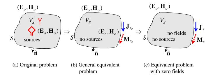
The equivalent problem in (b) assumes that the field inside the volume enclosed by S is given by  $(\mathbf{E}_e, \mathbf{H}_e)$ , which is different from the original field  $(\mathbf{E}_o, \mathbf{H}_o)$ . This results in a field discontinuity at the surface S, which demands the existence of surface current densities (as per Maxwell's equations):
