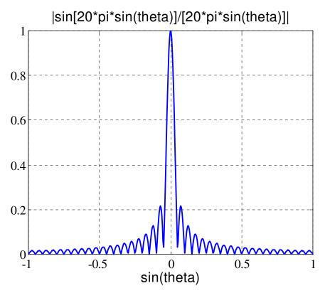
Here is a view of the  $|\sin v/v|$  function for  $L_y = 10\lambda$  and  $\varphi = 90^{\circ}$  (*E*-plane pattern):
