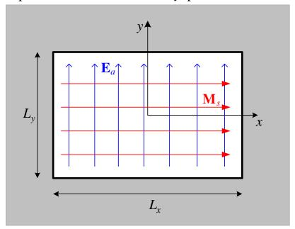
If the field is uniform in amplitude and phase across the aperture, it is referred to as a *uniform rectangular aperture*. Let us assume that the aperture field is *y*-polarized:
