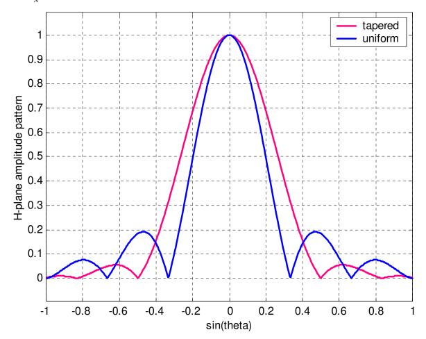
The above example of  $L_x = 3\lambda$  illustrates well the effect of source distribution on the far-field pattern. However, a more practical example is the rectangular-waveguide open-end aperture, where the waveguide operates in a dominant mode, i.e.  $\lambda_0 / 2 < L_x < \lambda_0$ . Here,  $\lambda_0$  is the wavelength in open space. Consider the case  $L_x = 0.75\lambda_0$ . The principal-plane patterns for an aperture on a ground plane look like this:
