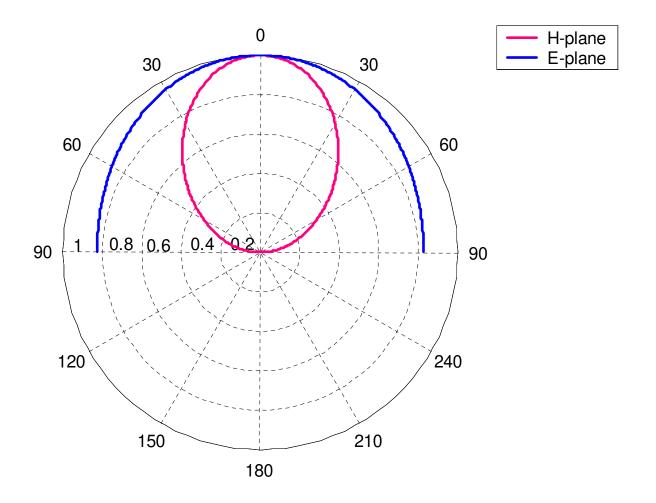
In the plot above, the polar patterns are shown for an X-band waveguide of cross-section defined by  $L_x = 2.286$  cm,  $L_y = 1.016$  cm. The frequency  $f_0 = 9.84$  GHz is considered when the free-space wavelength is  $\lambda_0 = 3.048$  cm.
