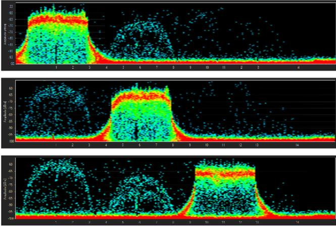
Fig. 6. Power Spectral Densities for 3 Orthogonal channels in the 802.11n 2.4 GHz band.
