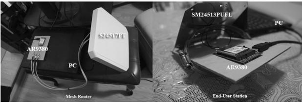
Fig. 4. WMN node configurations.
