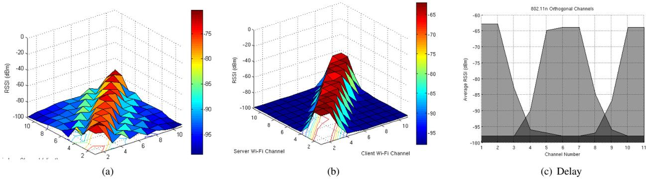
Fig. 7. (a) Mesh plot of 802.11b RSSI, (b) Mesh plot of 802.11n RSSI, (c) co-channel interference, channels 1, 6 and 11.
