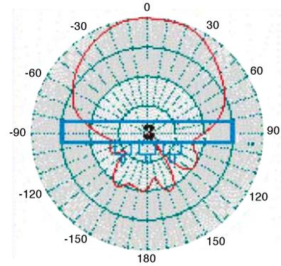
Fig. 5. 3x3 MIMO directional antenna radiation pattern.
