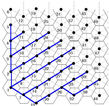
Fig. 1. A Wireless Mesh Network of 802.11n wireless routers supporting a backhaul tree (bold edges).
