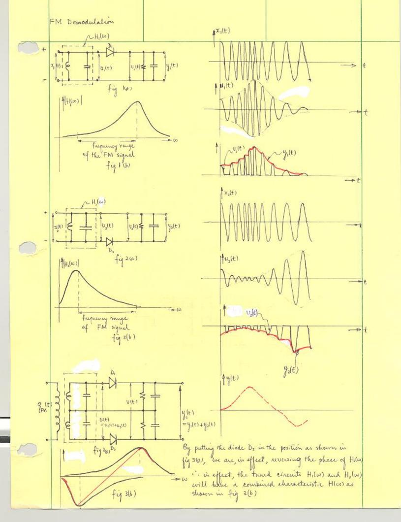
Note that the combined characteristic of H,(w) and H2(w) and onch as shown in fig 3(b) only when the diodes D4 and D2 are taken into account, ie, the prairies has been accounted for,
