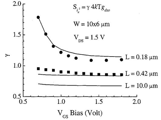
Fig. 4. Extracted (symbols) and simulated (lines)  $\gamma$  versus  $V_{GS}$  characteristics of the n-type MOSFETs with channel width  $W = 10 \times 6 \mu\text{m}$  and channel lengths  $L = 10 \mu\text{m}$ ,  $0.42 \mu\text{m}$  and  $0.18 \mu\text{m}$ , respectively, biased at  $V_{DS} = 1.5 \text{ V}$  with  $\delta = 0$ .
