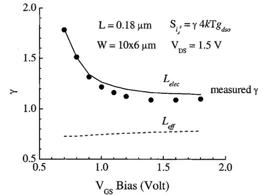
Fig. 5. Extracted (symbols) and simulated (lines)  $\gamma$  versus  $V_{GS}$  characteristics of the n-type NMOSFET with channel length  $L = 0.18 \mu\text{m}$  and width  $W = 10 \times 6 \mu\text{m}$  and biased at  $V_{DS} = 1.5 \text{ V}$  with  $\delta = 0$ . The solid lines are obtained by using  $L_{elec}$ , and the dashed lines are obtained by using  $L_{eff}$  in (11).
