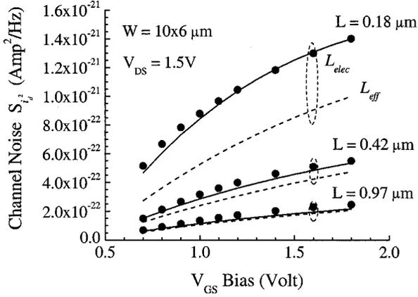
Fig. 2. Extracted (symbols) and simulated (lines) spectral density of the channel noise versus  $V_{GS}$  characteristics of the n-type MOSFETs with channel width  $W = 10 \times 6 \mu\text{m}$  and channel lengths  $L = 0.97 \mu\text{m}$ ,  $0.42 \mu\text{m}$  and  $0.18 \mu\text{m}$ , respectively, biased at  $V_{DS} = 1.5 \text{ V}$  with  $\delta = 0$ . The solid lines are obtained by using  $L_{elec}$  and the dashed lines are obtained by using  $L_{eff}$  in (11).
