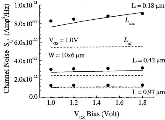
Fig. 3. Extracted (symbols) and simulated (lines) spectral density of the channel noise versus  $V_{DS}$  characteristics of the n-type MOSFETs with channel width  $W = 10 \times 6 \mu\text{m}$  and channel lengths  $L = 0.97 \mu\text{m}$ ,  $0.42 \mu\text{m}$  and  $0.18 \mu\text{m}$ , respectively, biased at  $V_{GS} = 1.0 \text{ V}$  with  $\delta = 0$ . The solid lines are obtained by using  $L_{elec}$  and the dashed lines are obtained by using  $L_{eff}$  in (11).
