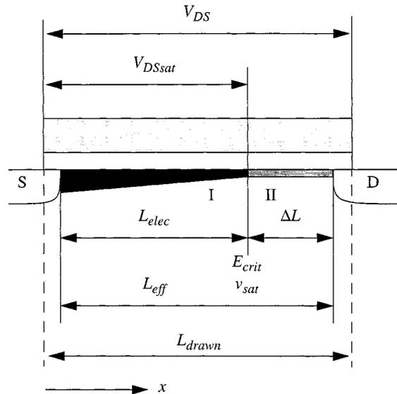
Fig. 1. Cross section of a MOSFET channel divided into a gradual channel region (I) and a velocity saturation region (II).
