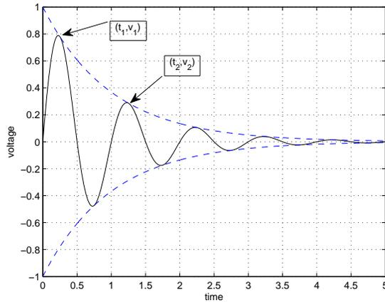
Figure 1: A voltage in an under-damped circuit.
