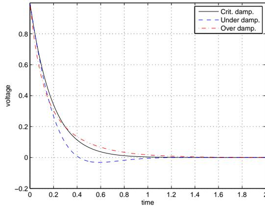
Figure 2: A voltage in critically-damped, under-damped and over-damped versions of a circuit.
