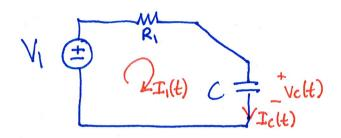
$$\Rightarrow \frac{dV_{clt}}{dt} + \frac{V_{clt}}{R_{i}C} = \frac{V_{i}}{R_{i}C}$$
