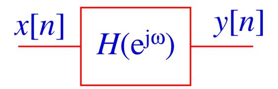
The impulse response values  $\{h[0], h[1], h[2], ...\}$  can be interpreted as filter coefficients.
