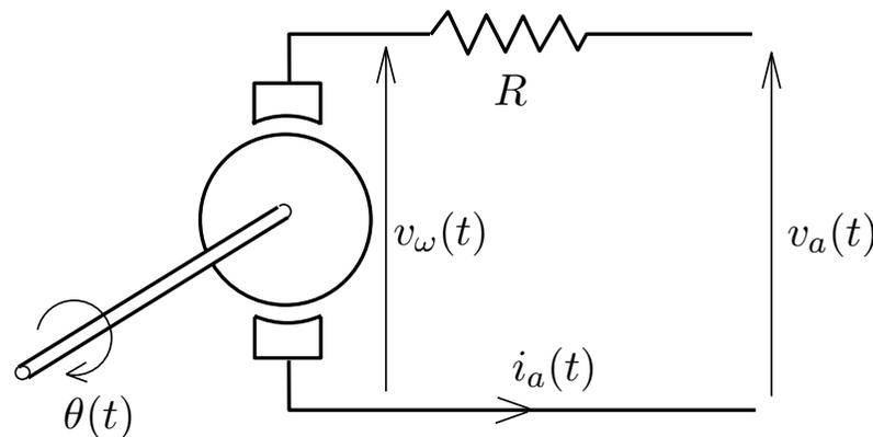
Figure 3.2: *Simplified model of a d.c. motor*
