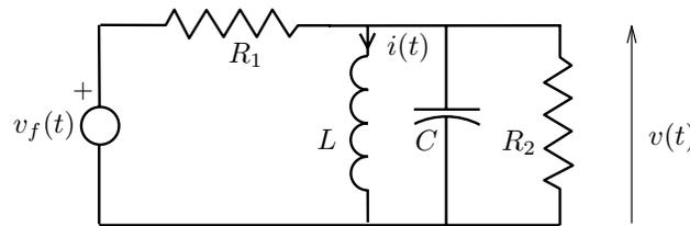
Figure 3.1: *Electrical network. State space model.*
